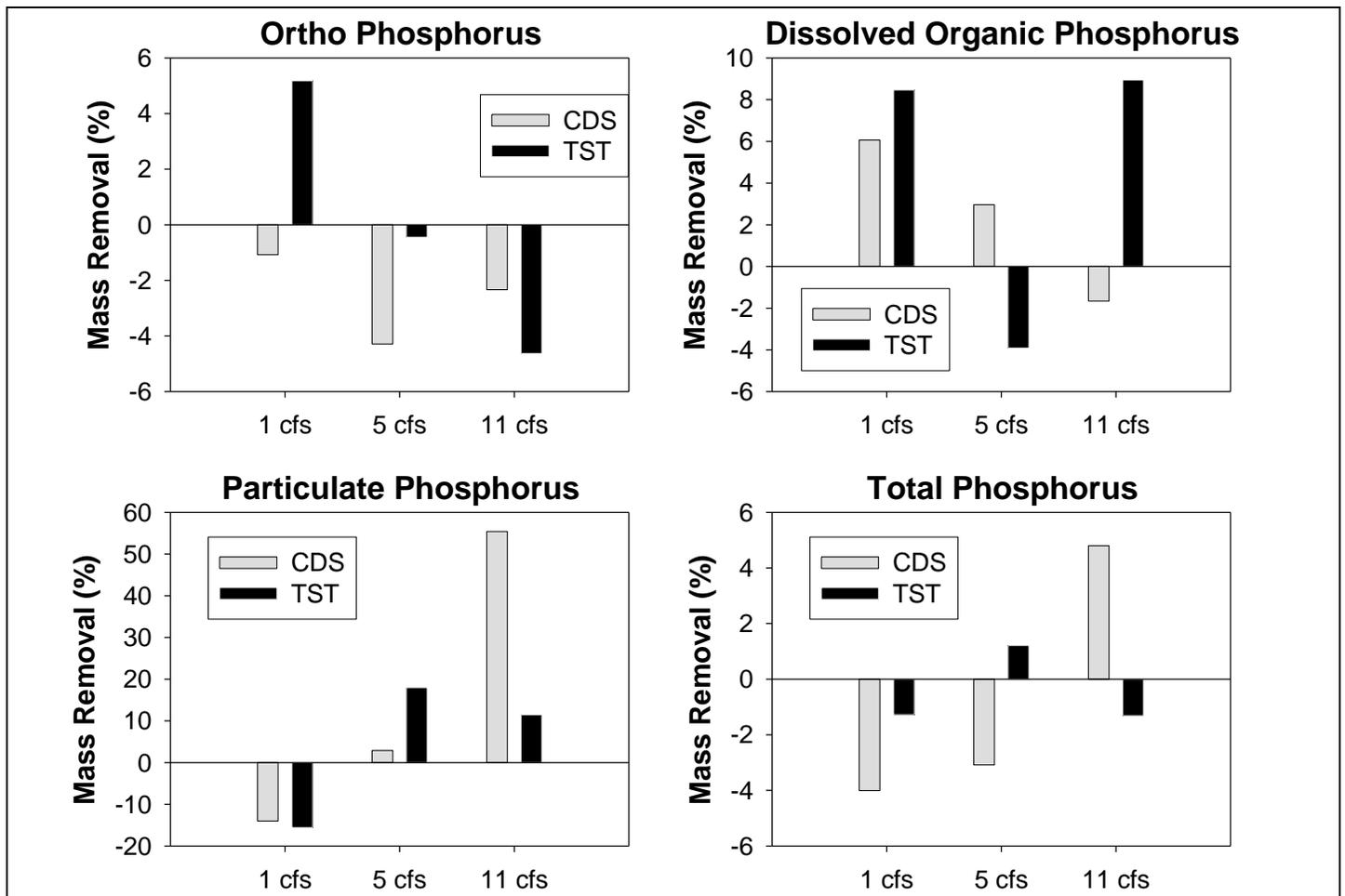
Figure 7. Comparative Mass Removal Efficiencies for Phosphorus Species in the CDS and TST Units.
