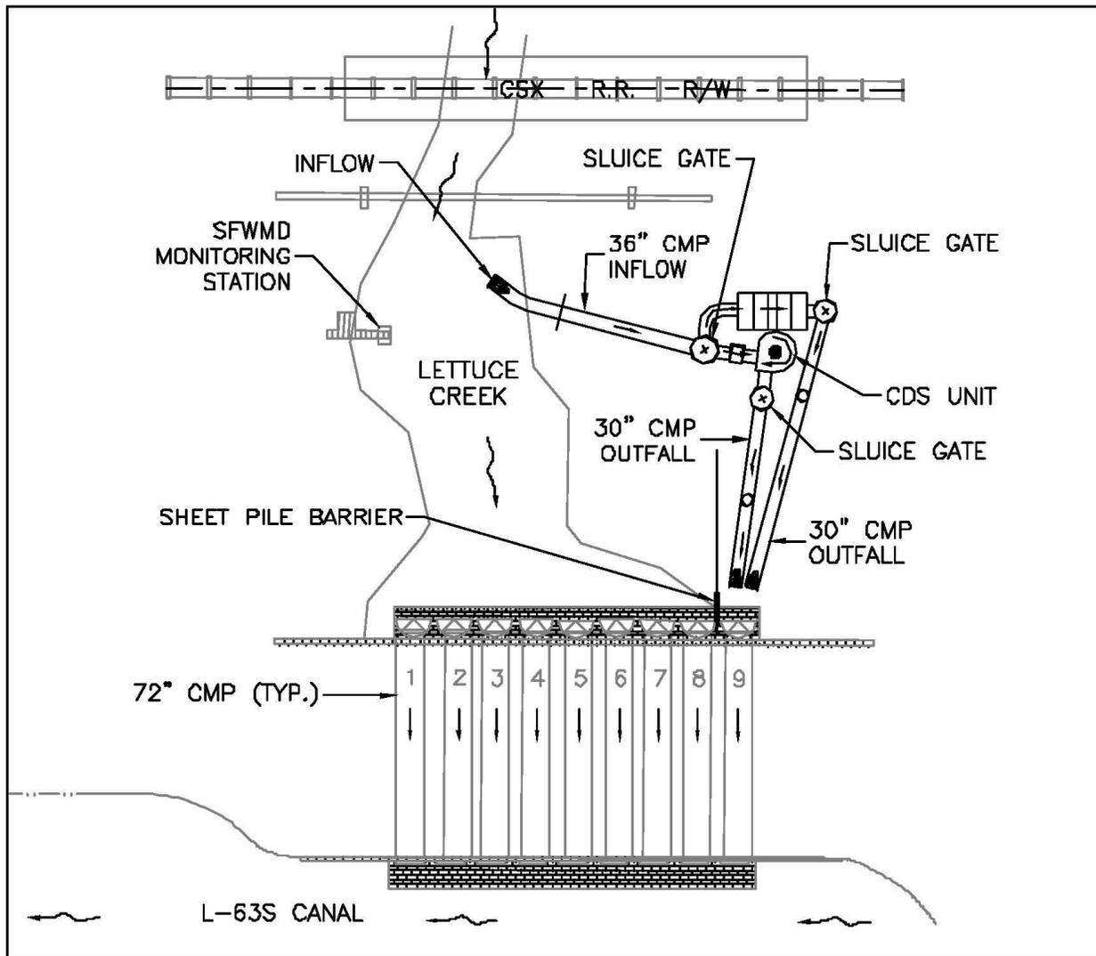
Figure 2. Plan View of the CDS and TST Unit Installation.
