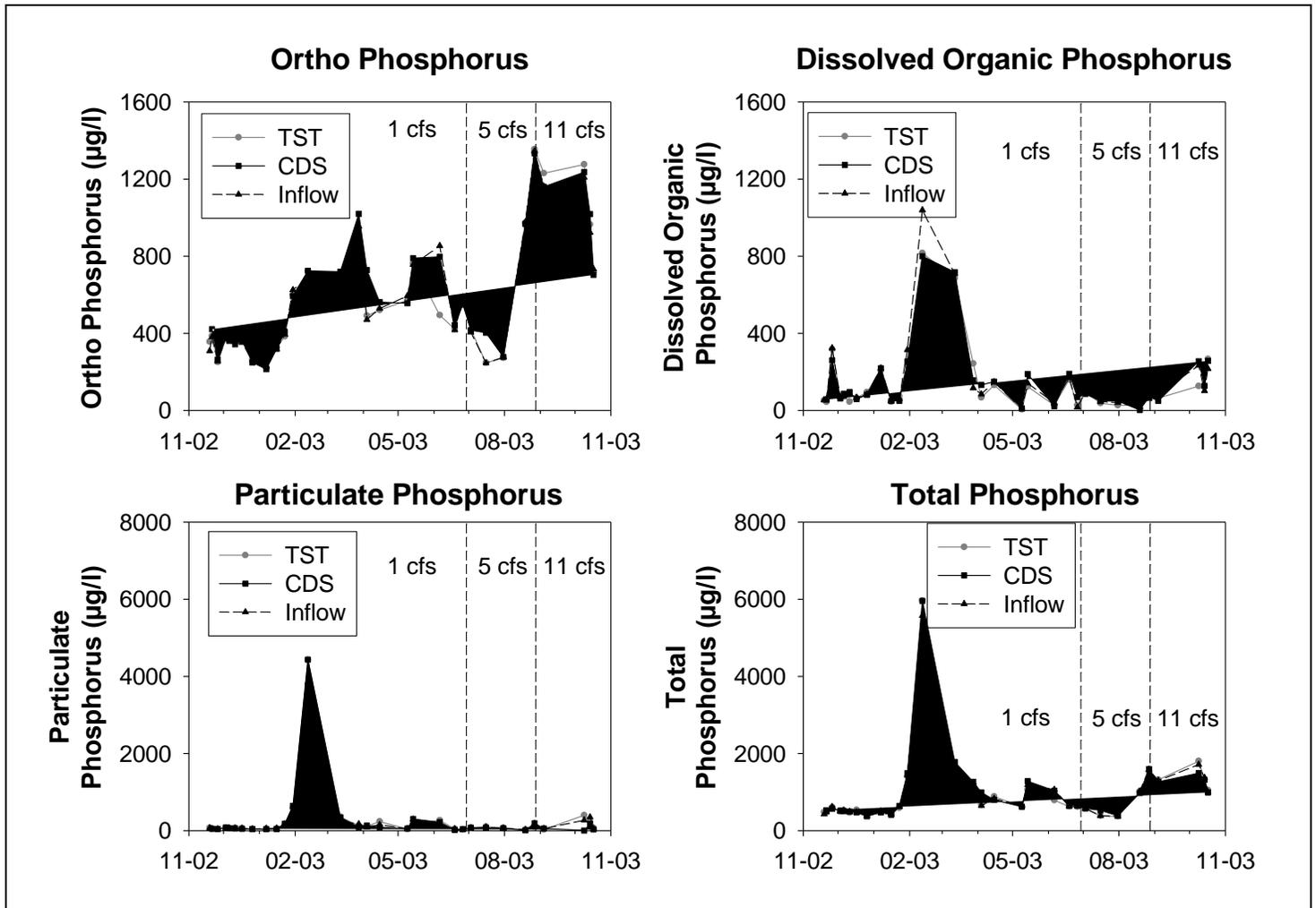
Figure 6. Concentrations of Phosphorus Species in Inflow and Outflow of the CDS and TST Units.
